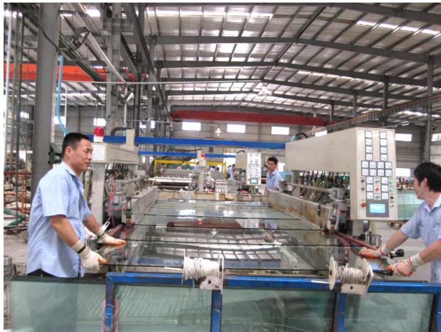
▲ New double edger for flat polishing
